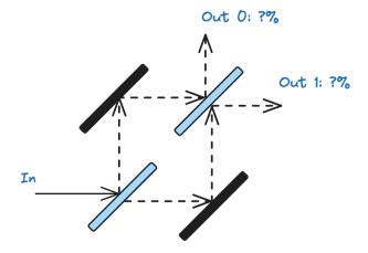
It turns out that the beam splitter acts like a Hadamard gate, and the horizontal "input" is like a  $|0\rangle$  state, and the vertical "input" is like a  $|1\rangle$  state.
